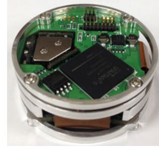
Fig. 2. Shape of the MEMS ISA.
