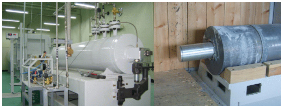
Fig. 16. High-impact gas-gun tester.
