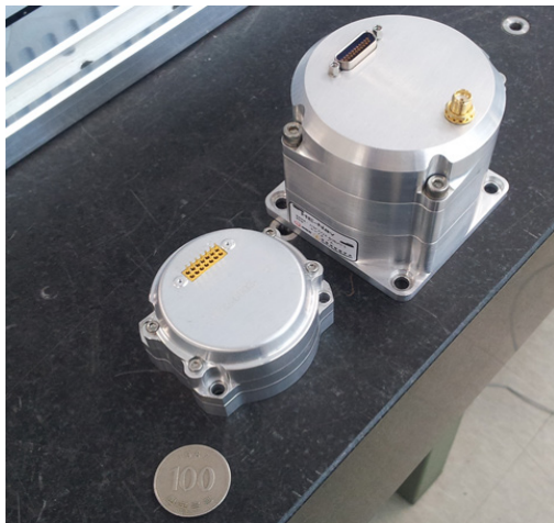
Fig. 10. Shape of the MEMS-IMU/GPS integrated navigation system.
