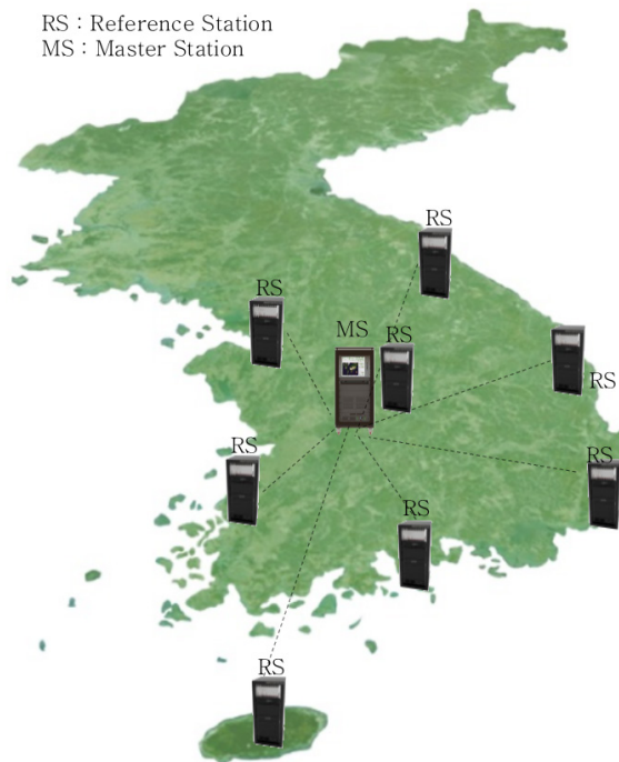
Fig. 1. System architecture of ADD WADGPS testbed.
