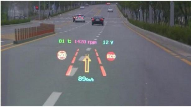
Fig. 3. Mismatch between AR-based contents and road in a HUD-based navigation system.
