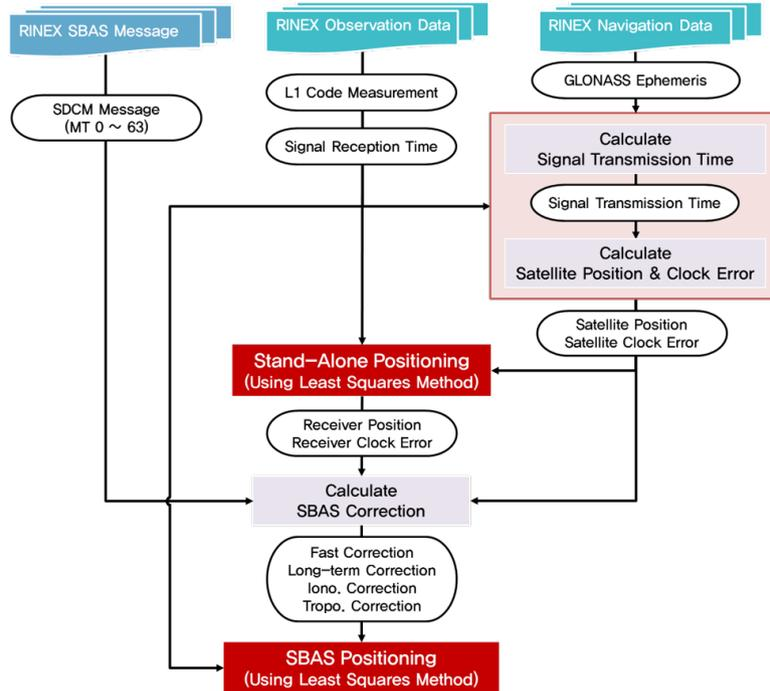
Fig. 3. SBAS positioning algorithm using SDCM corrections.
