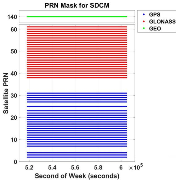
Fig. 2. PRN mask for MT 1 transmitted by SDCM.
