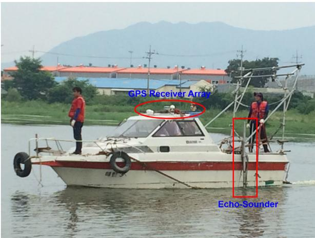
Fig. 6. Survey boat equipped with GPS receivers and eco-sounder.
