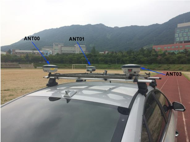
Fig. 5. GPS receivers on roof of trial vehicle.
