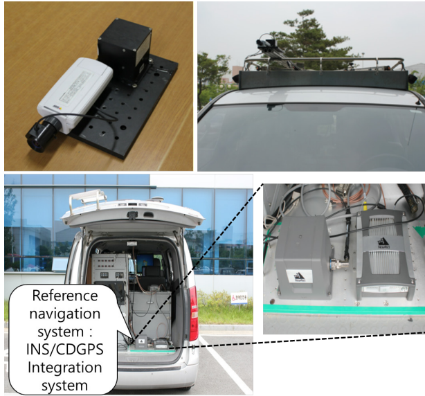
Fig. 11. Experimental setup and reference navigation system.
