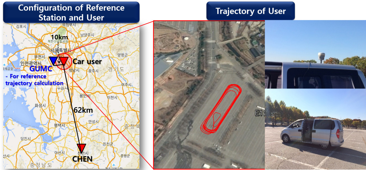
Fig. 3. Test configuration for performance validation of medium-baseline RTK.
