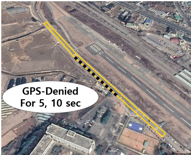
Fig. 7. Experiment area and artificially generated GPS-denied environment.
