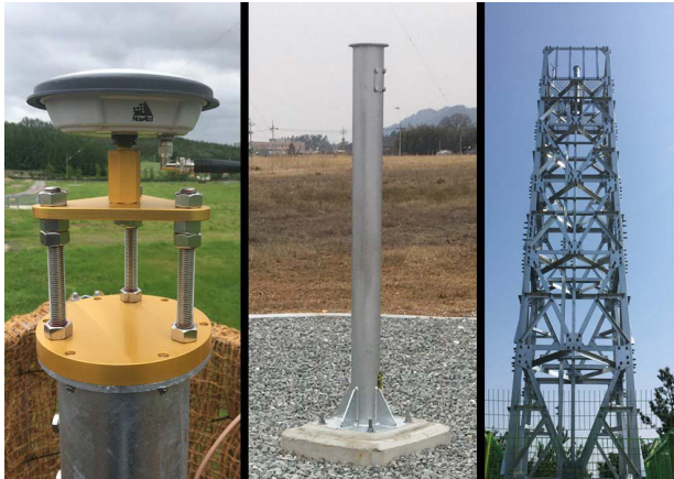
Fig. 6. GPS adapter, steel pipe, steel tower.
