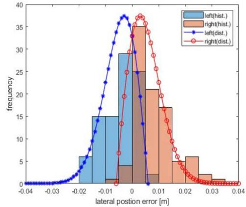
Fig. 2. Distribution of the lateral position error in one step.
