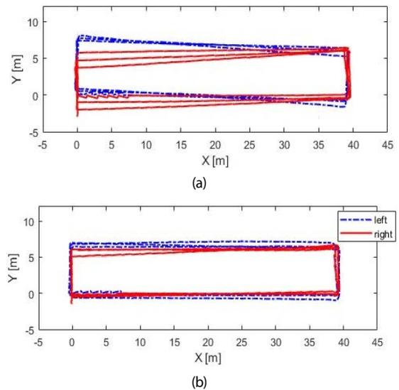
Fig. 8. Estimated position using each algorithm (square trajectory). (a) standalone PDR. (b) proposed DF-PDR system.
