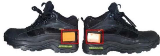
Fig. 5. Location of the inertial sensors.
