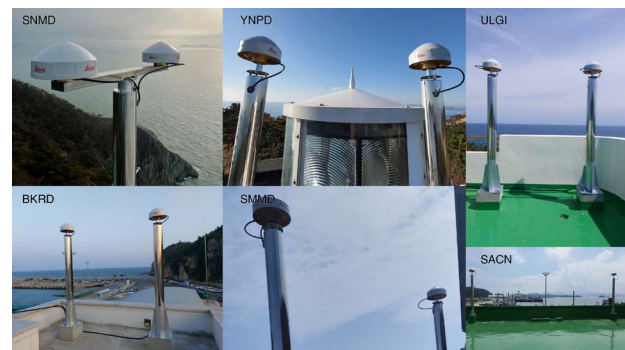
Fig. 4. Installed GNSS antennas at POINT reference stations: SNMD (top left), YNPD (top middle), ULGI (top right), BKRD (bottom left), SMMD (bottom middle), and SACN (bottom right).
