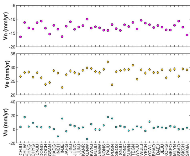
Fig. 3. The magnitude of the GNSS velocity vector by the north, east, and up directions for all stations.
