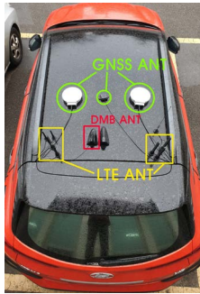
Fig. 9. Test road – mobile positioning system antenna setup.
