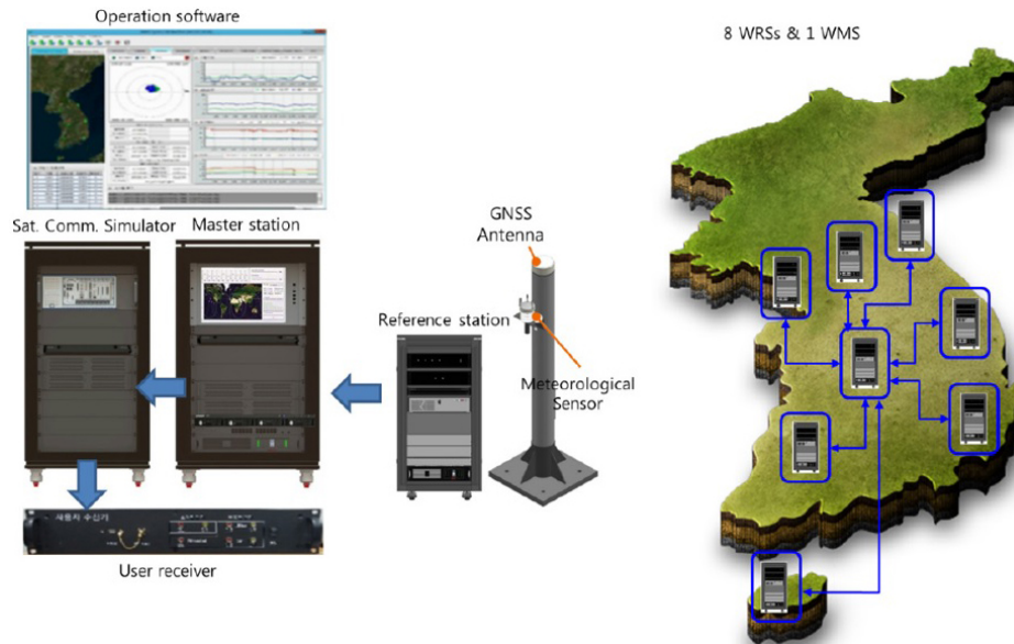
Fig. 1. Conceptual view of WADGPS testbed (So et al. 2016a).
