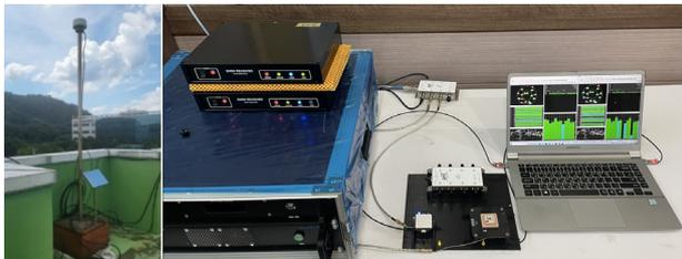
**Fig. 2.** GNSS & SBAS (KASS) signal test bed setup using commercial receiver.
