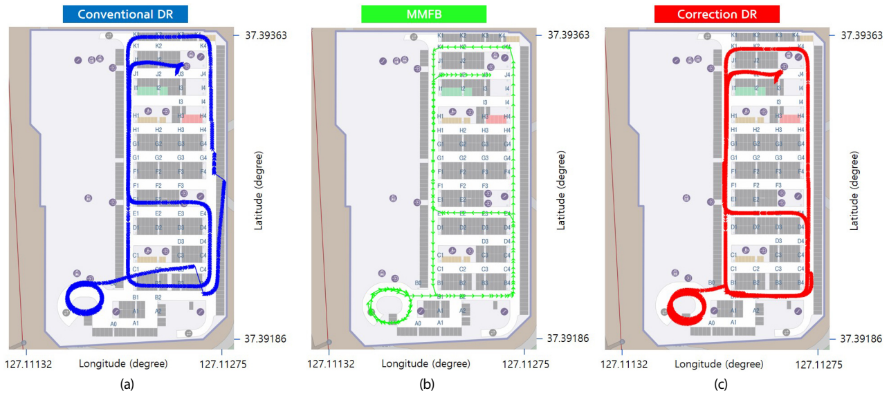
Fig. 8. Comparison of Conventional DR and proposed CDR positioning performance in an underground parking lot (STD5W AVN, (a) Conventional DR result in scenario #1, (b) MMFB result in scenario #1, (c) Correction DR result in scenario #1).
