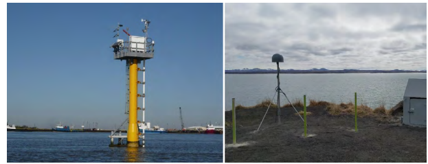
Fig. 4. Photos of GNSS-R experimental stations installed at coastal sites with open visibility to the sea surface: (left) CALC station in Louisiana, (right) AT01 station in Alaska.
