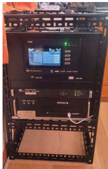
Fig. 4. Ship-mounted VDES R-Mode receiver and reception server.
